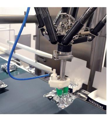
The high-speed, flexible, patent-pending Peregrine<sup>™</sup> from JLS Automation is ideal for the hygienic and efficient loading of frozen foods into tri-seal and other cartons. It utilizes a proprietary positive carton transport (PCT) system to retain full control of the carton from forming through loading, without ever letting go.
